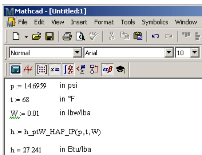
**Figure 2.3.4:** Example Mathcad® sheet with finished calculation
