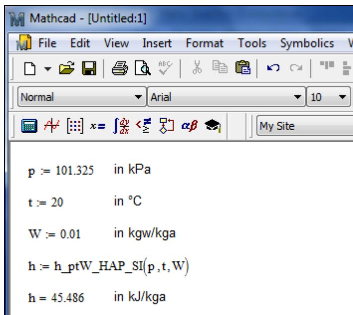
**Figure 2.2.4:** Example Mathcad® sheet with finished calculation
